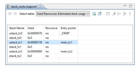
As you can see, apart from the default ustack\_tc0 and istack\_tc0, there are now also stack estimations for the stacks ustack\_tc1 and ustack\_tc2. These entry points are now also visible in the call graph as root functions.
