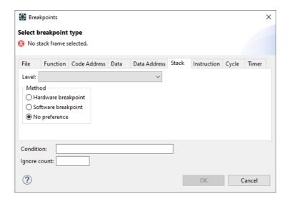
The target halts when it reaches the specified stack level.
