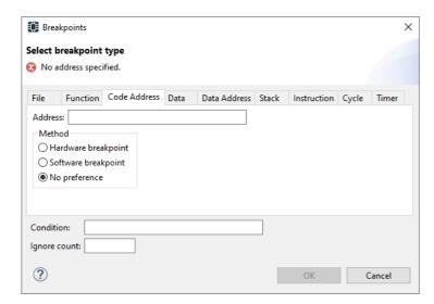
The target halts when it reaches the specified instruction address.
