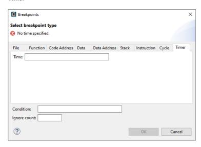
The target halts when the given amount of **Time** elapsed. The value entered is interpreted by the debug instrument.
