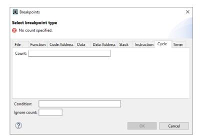
The target halts when the given number of clock cycles (Count) has elapsed.
