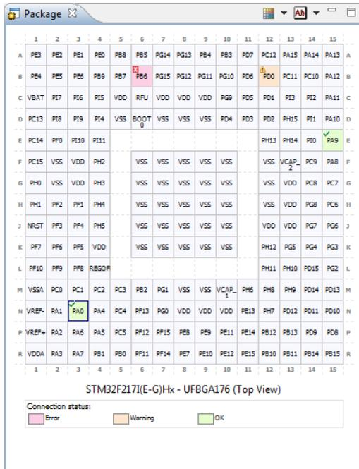
A square around a pin marks the selected pin. In the package above PA0 is selected. A green check mark indicates that the pin has a valid connection; PA0 and PA9 in the package above. A red cross indicates an error; PB6 in the package above. A triangle with exclamation mark indicates a warning; PD0 in the package above. When you click on a pin, the pin appears in the editor. If the pin contains an error, you can see what is wrong in the Pin Conflicts view.
