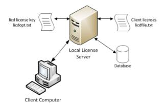
In this situation, the local license server licenses itself by reading its license data from a local key. This key must be obtained from TASKING support and added to licdopt.txt.
